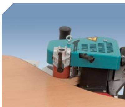
Easy banding of shaped and round panels.
